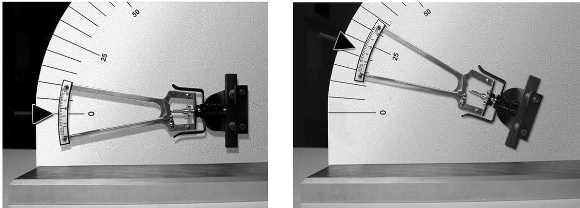
Figure 2: Left: Tonometer in the horizontal position with the plunger in the upper position, indication below the scale value 0.
