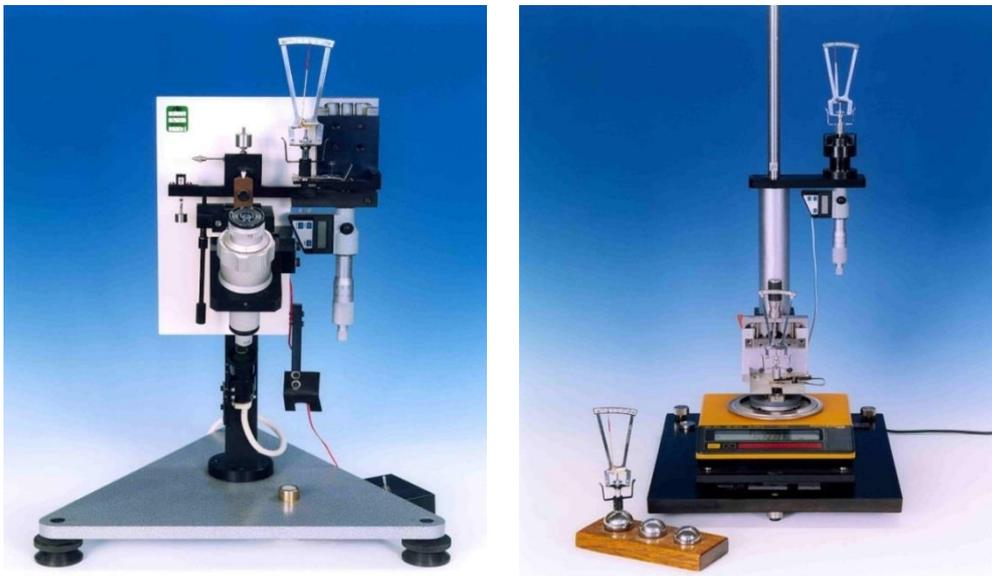
*Figure 1: Test equipment used for the verification of impression tonometers.*
