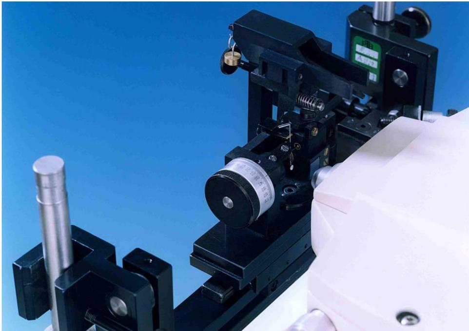
*Figure 4: PTB-jig (flapper) for the metrological verification of non-contact tonometers*
