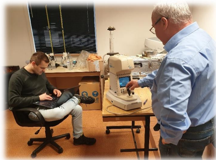
Fig. 2: Measurement using standard device - eye model - at the Czech Metrology Institute
